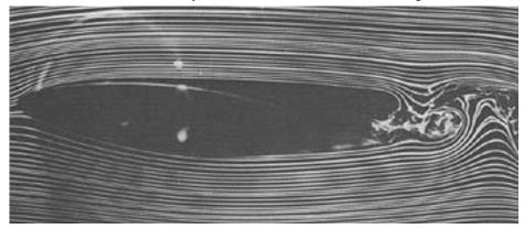
Figure 1. Streamlines of smoke around an airplane wing in a wind tunnel. (*Image source*: NASA, http://history.nasa.gov/SP-4103/app-f.htm)
