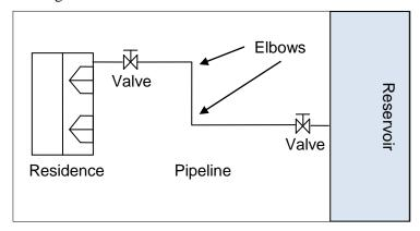
Figure 2. Pipeline from a reservoir to a single residence.
