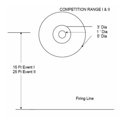
Mentor Note: Target may be constructed as follows: Bulls Eye—use a pie tin taped down. The diameter is approximately 1' and when it hits it "pings", which increases the thrill of the team able to acquire a direct hit. Middle and Outer rings—use  $\frac{1}{4}$ " tubing, string, or rope lengths of 15.7' and 9.4' to form circles. Join ends of tubing with a  $\frac{1}{4}$  wood dowel as a plug. Tape tubes to the floor. Buckets as bullseyes can also make a nice target.
