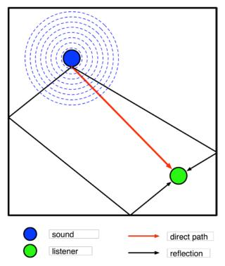
Notice in the diagram above that as the sound waves propagate from the sound source, some of the sound waves bounce off of the walls (NOTE: Only two paths are shown for the reflection waves, but many more exist as the wave propagates in all directions from the sound source as is seen by the blue dashed lines).
