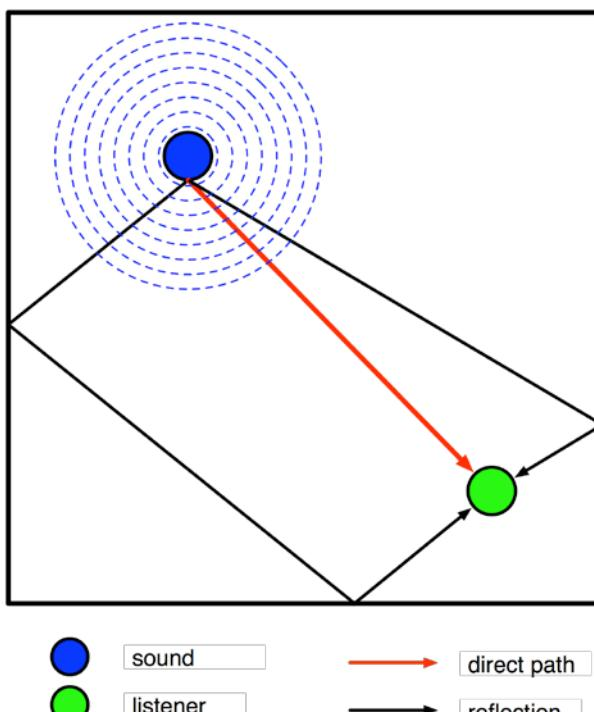
Notice in the diagram above that as the sound waves propagate from the sound source, some of the sound waves bounce off of the walls (NOTE: Only two paths are shown for the reflection waves, but many more exist as the wave propagates in all directions from the sound source as is seen by the blue dashed lines).
