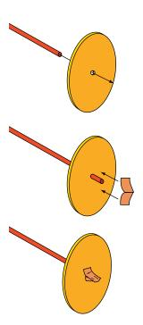
**3.** Cut two large straws to the size you want. Tape them parallel to each other on the bottom of the racer body at opposite ends. Slide a wheel and axel through one of the straws and mount a second wheel on the other end of the axle.
